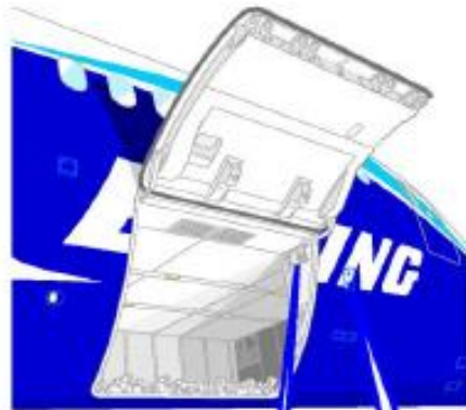
Fwd Cargo Compartment (Aft Similar)
