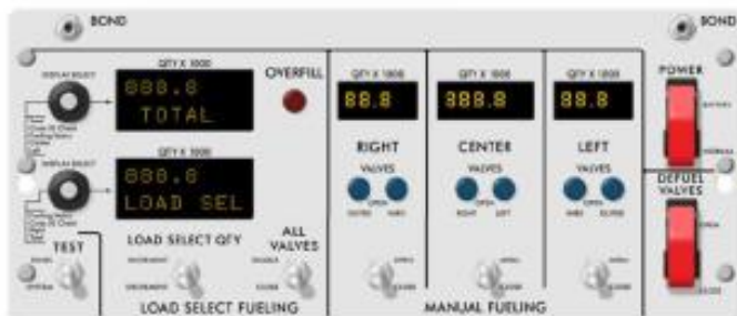
Refuel Control Panel (RCP)
