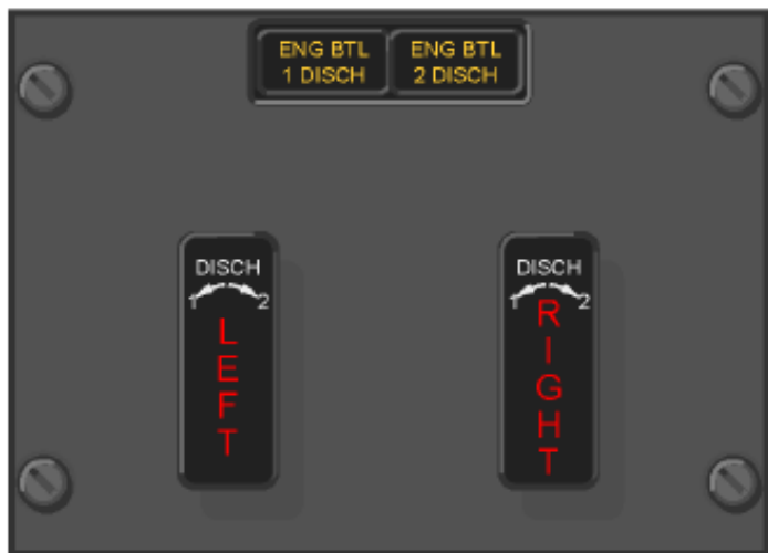
Engine Fire Control Panel
