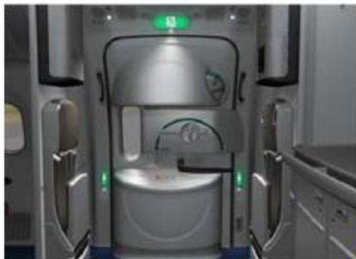
Exit Identifier/Exit Marking Sign
